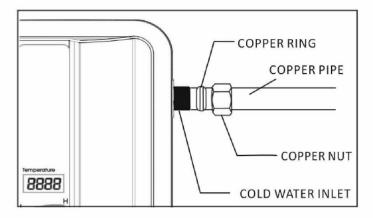
This water heater is supplied with 1/2" compression fittings, Do not weld or use Teflon or paste.
