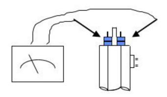
If the reading is less than 20 ohms on the "Rx 1" scale or the "Rx 10" scale the element is good, if it is much greater e.g.... 10,000 ohms or if you get a reading on the "Rx 1K" scale then you must replace the element (contact Eemax). Tel: 1-800-543-6163 for replacement elements. (Please note down the resistance value if you need to contact Eemax; This will be very useful to us.)
