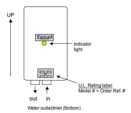
This is how your Eemax "EX-T" model should look when mounted correctly on the wall.
