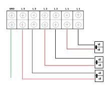
DISCONNECT ALL BREAKERS AT THE SERVICE PANEL. ONCE ALL BREAKERS HAVE BEEN DISCONNECTED MEASURE THE VOLTAGE GOING TO EACH ONE OF THE SETS (L1 L1) (L2 L2) (L3 L3) ALL SHOULD READ 0 VOLTAGE.
