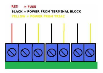
CHECK THE FUSE USING YOUR VOLT METER. PLACE ONE PROBE ON THE FARTHEST LEFT TERMINAL BLOCK THAT HAS THE **RED** FUSE WIRE CONNECTION AND THE OTHER PROBE TO GROUND. YOU SHOULD GET A VOLTAGE READING OF 110-120V, IF THERE IS NO READING THE FUSE MUST BE REPLACED.
