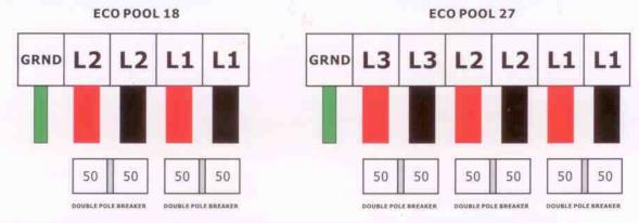
Wire & Breakers specification based on the model being installed
