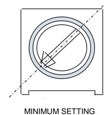
THE TEMPERATURE CONTROLLING POTENTIOMETER IS A PRECISION COMPONENT. ADJUST GENTLY AND DO NOT TURN BEYOND THE MIN. AND MAX. STOP POINTS
