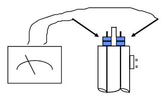
If the reading is less than 20 ohms on the "Rx 1" scale or the "Rx 10" scale the element is good, if it is <u>much</u> greater e.g.... 10,000 ohms or if you get a reading on the "Rx 1K" scale then you must replace the element (contact Eemax). Tel : 1-800-543-6163 for replacement elements. (Please note down the resistance value if you need to contact Eemax; This will be very useful to us.)
