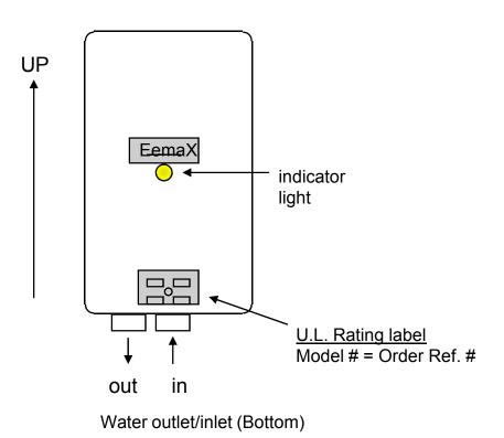
This is how your Eemax "EX" models should look when mounted correctly on the wall.
