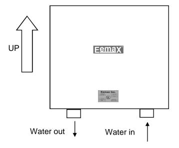
This is how your Eemax "Series Two" water heater should look when correctly mounted on the wall. <u>ANY</u> other mounting configuration is wrong and the unit will <u>NOT</u> work!
