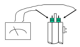
If the reading is less then 20 ohms on the single (Rx 1) or (Rx 10) scale, then the element is good, if it is much greater e.g. 10,000 Ohms or a reading with a small M or K next to it, you will need to change the element. To do this, contact Eemax, 1-800-543-6163, and report the tests you have performed. Be ready to give the order ref number and serial number for your heater.
